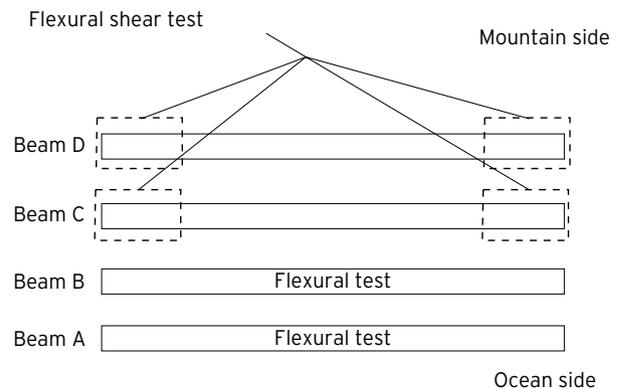
Figure 2. Loading types and positions
