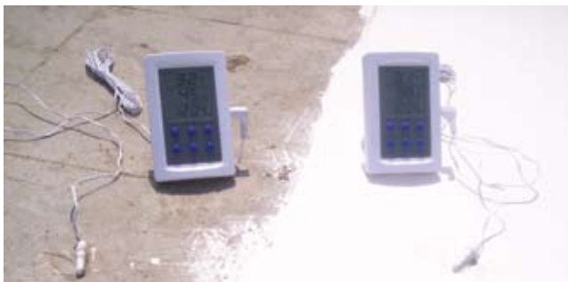
Fig. 2: Measurement of temperature difference between Energy Efficient Heatshield coated and uncoated surfaces
