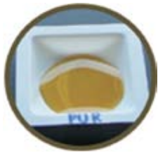
Fig. 7a: PU healing agent before polymerization
