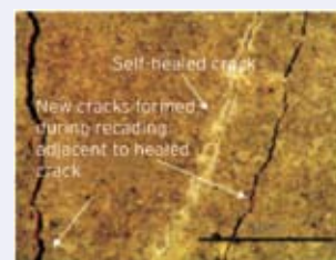
Fig. 4: Cracks through virgin ECC material adjacent to a self-healed crack held tight by self-healing material
