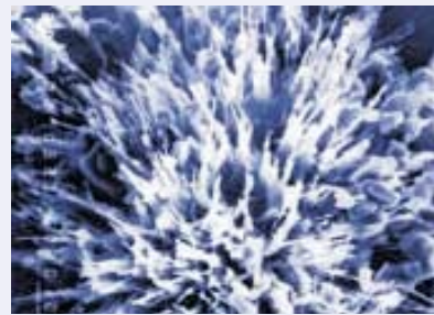
Fig. 2: Crystallization being formed for blocking capillaries
