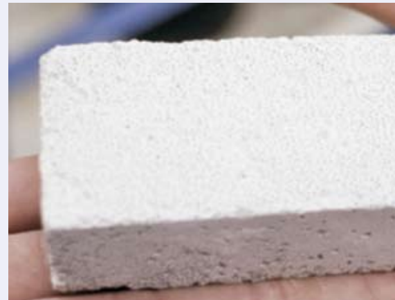
Fig. 3: Concrete matrix embedded with a micro-encapsulated sodium silicate healing agent
