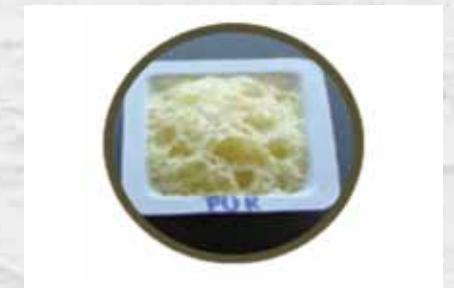
Fig.1b PU healing agent after polymerisation
