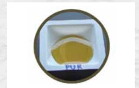
Fig.1a PU healing agent before polymerisation
