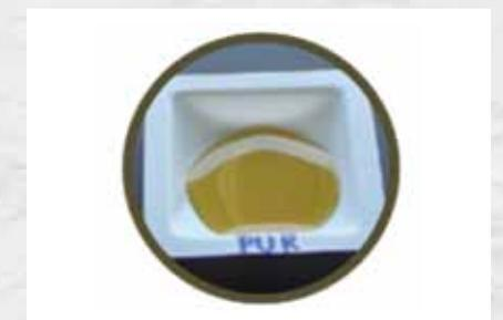
Fig.1a PU healing agent before polymerisation
