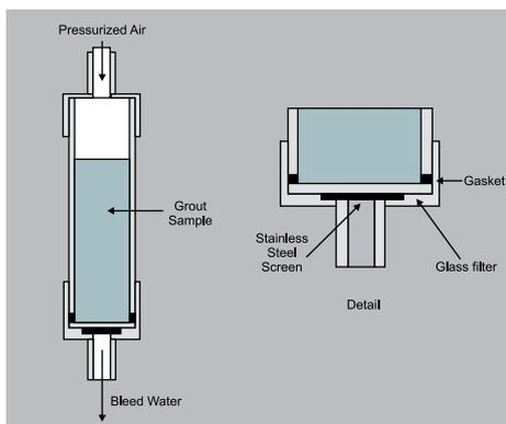
Figure 3 - Bleed Under Pressure Test (Gelman Filtration Funnel)
