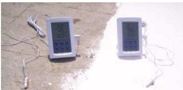
**Fig. 2:** Measurement of temperature difference between Energy Efficient Heatshield coated and uncoated surfaces. Some of the other facets of green buildings are: heat reduction insulated roofs (Fig. 2) and walls that substantially reduce heat ingress (up to 60%) thereby resulting in lower AC loads, cross ventilation with fresh breeze, goodbye
