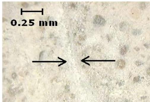
Fig. 5: Crack repaired with bacteria in Sol-gel medium
