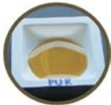
**Fig. 7a:** PU healing agent before polymerization
