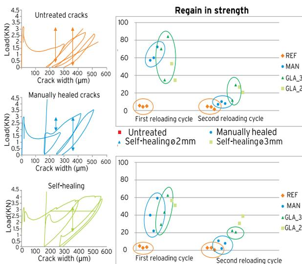
**Fig. 8:** Regain in mechanical properties due to crack-healing
