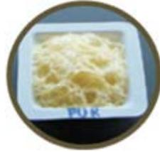
**Fig. 7b:** PU healing agent after polymerization
