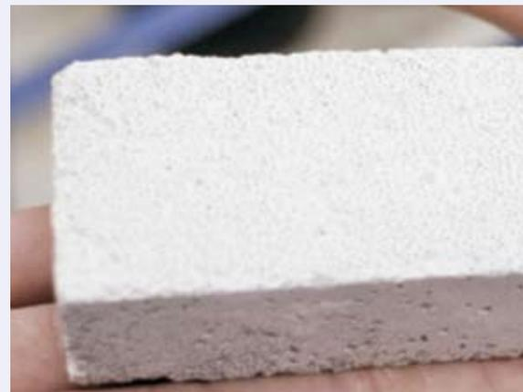
Fig. 3: Concrete matrix embedded with a micro-encapsulated sodium silicate healing agent
