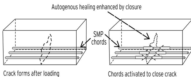
Fig.2: Shape-memory polymer-cementitious composite
