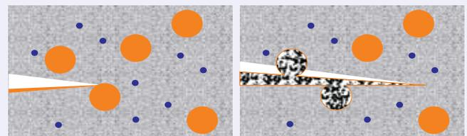
Fig. 1: Depiction of crack propagation through microcapsule-embedded material
