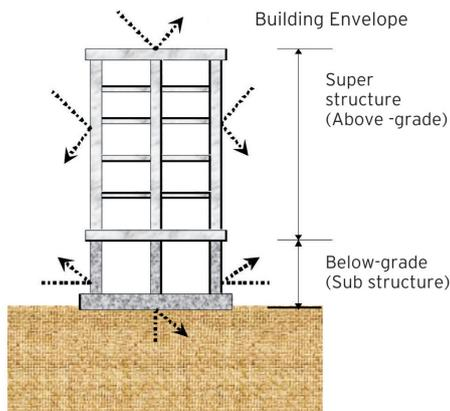
Fig. 2: Schematic diagram of building envelope
