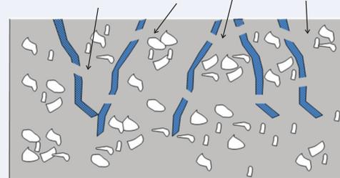
Fig. 1: Integral Water Proofers - Pore Blocking Effects
