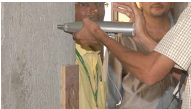
Fig. 1: Testing of rebound hammer on concrete surface
