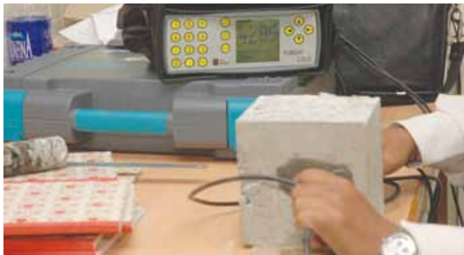
Fig. 1: Testing of ultrasonic pulse velocity of a concrete cube
