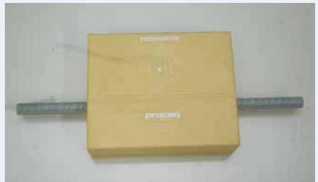
Fig. 2: Calibration block of Profometer
