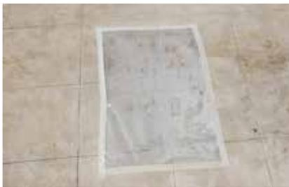
**Fig. 16c:** Checking the moisture content of the substrate by enclosing with polythene sheet
