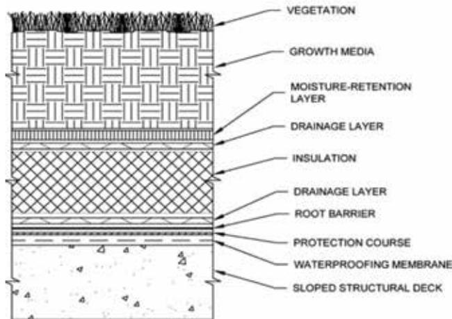
**Fig. 3 :** A vegetative roof system with an inverted assembly and drainage layers above and below the insulation
