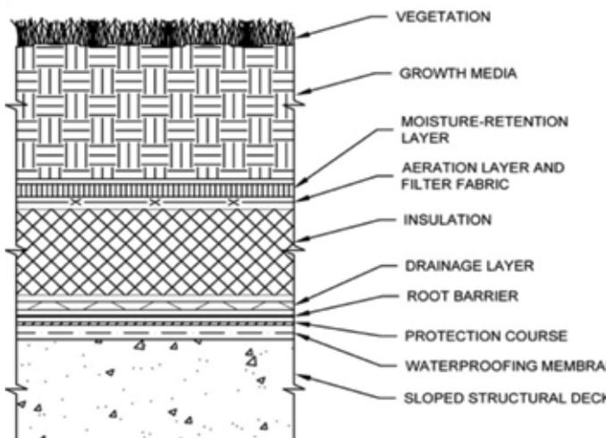
**Fig. 1 :** A vegetative roof system with an inverted assembly (The position of the root barrier varies by design)
