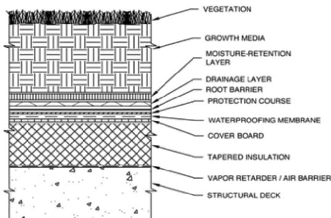
**Fig. 2 :** A conventional roof assembly adapted to a vegetative roof system
