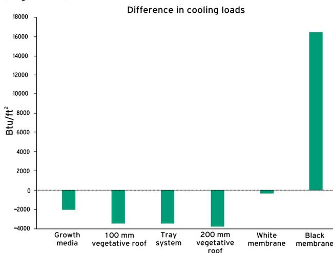
**Fig. 6 :** A The SPRI/ORNL vegetative roof study measured cooling loads of vegetative and black roof sections indexed to the white section cooling load
