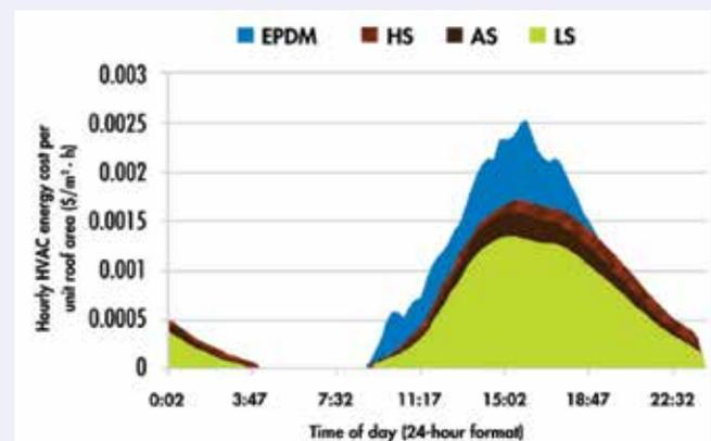
**Fig. 5 :** HVAC energy cost comparison
