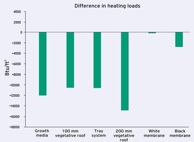
**Fig. 7 :** The SPRI/ORNL vegetative roof study measured heating loads of vegetative and black roof sections indexed to the white section heating load
