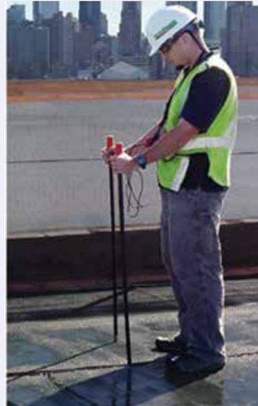
**Fig. 1:** In Low Voltage Vector Mapping (wet testing) the technician uses metal probes on a wet surface to pinpoint membrane breaches
