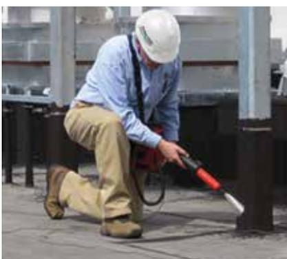
**Fig. 3:** ELD Fusion method of membrane integrity testing
