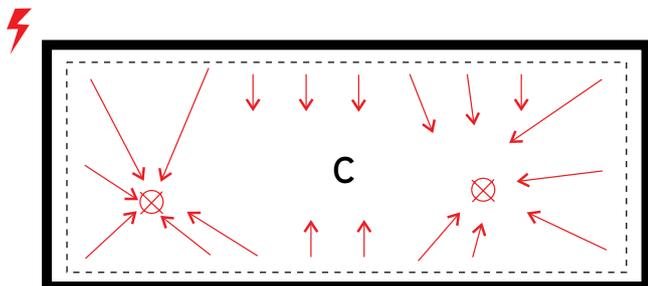
**C:** If the membrane is not watertight, the electricity makes a ground connection and is pulled toward positive poles.
