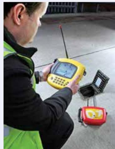
Fig. 4: Leakage detection by Digital leakage correlator
