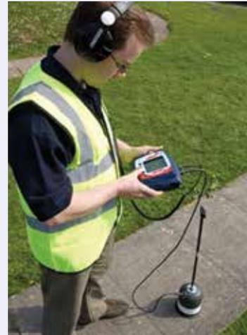
Fig. 3: Leakage detection by advanced Ground Microphones
