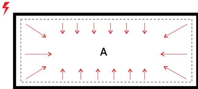
**A:** Small electrical pulses are directed onto the membrane. The electricity searches for a ground connection
