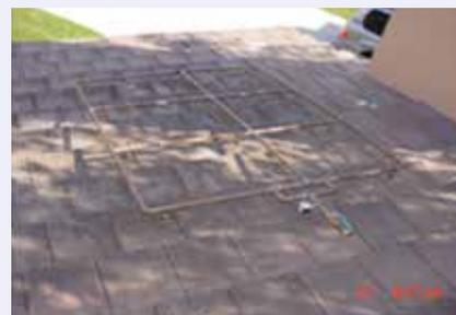
Fig. 13: Images of the spray rack system used to apply water to the roof
