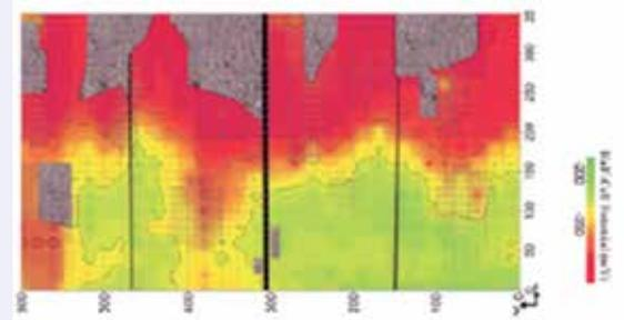
(a) Half-cell corrosion potentials
