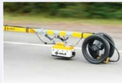
Fig. 12: GPR survey being used to evaluate the characteristics of road pavement
