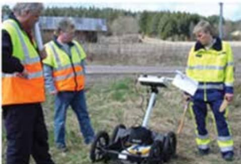
Fig. 4: GPR survey for detecting underground storage tank
