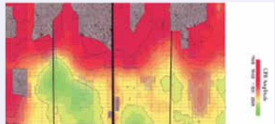
(b) GPR rebar level attenuation
