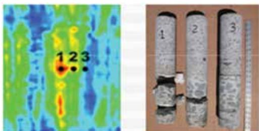
Fig. 7: Verification of concrete deterioration by GPR and core samples
