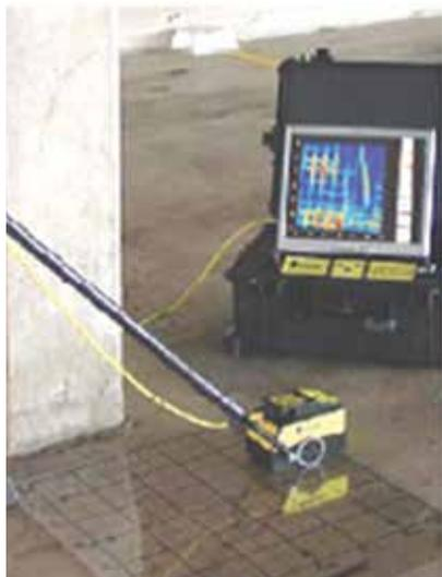
Fig. 2: A GPR survey for concrete structures
