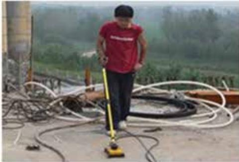
Fig. 8: GPR survey for locating embedded electrical conduits in concrete
