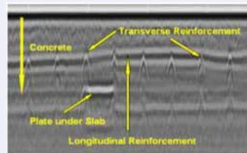
**Fig. 4:** Longitudinal and transverse reinforcing bars profiling during a GPR survey
