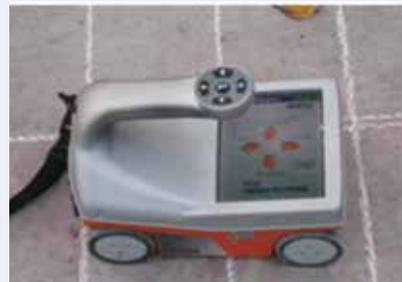
Fig. 3: Latest Model of GPR
