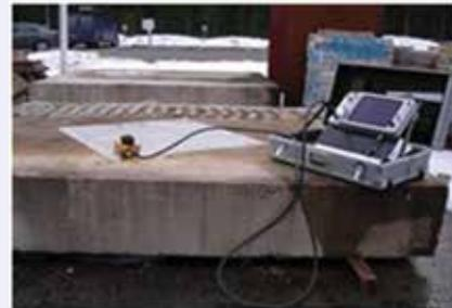
Fig. 11: GPR survey being used to evaluate the deterioration of RCC slab
