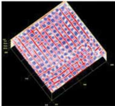
Fig. 5: C-scan - Reinforcements in a Slab
