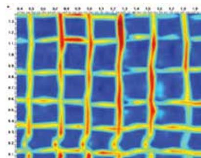
Fig. 1b: 2D horizontal plot of rebar array in RCC pavement collected by GPR
