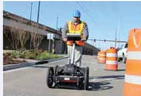
Fig. 1: GPR survey for locating utility services on a road
