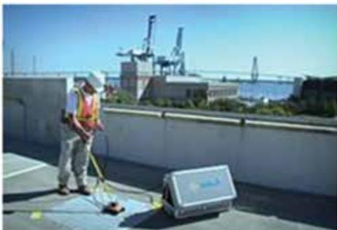
Fig. 9: GPR survey for detecting voids inside concrete
