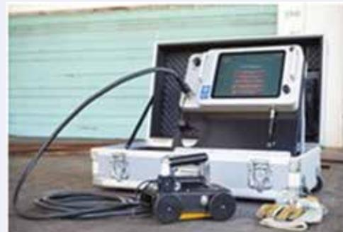
Fig. 6: GPR survey for locating post-pre- tension cables
