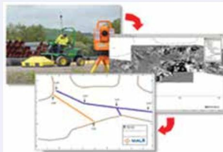
Fig. 2: GPR survey for utility mapping and their location mapping (bottom drawing) along with their 3D view of the location (top right)
