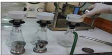
Fig. 8: Setup of Alkali Aggregate Reactivity Test for Aggregates by Chemical Method
