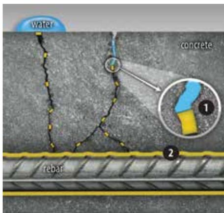
1. Hydrophobic pore blocking 2. Corrosion-inhibiting surface coating
