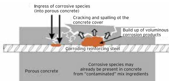
Fig. 1: Reinforcement corrosion process
