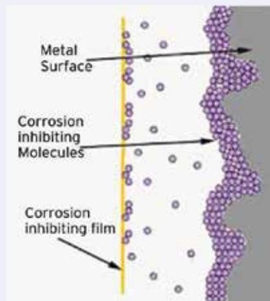
**Fig. 5:** Migration of corrosion inhibiting molecules
