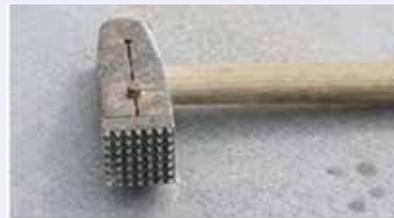
Fig. 10: View of a Bush hammer used for surface removal of concrete
