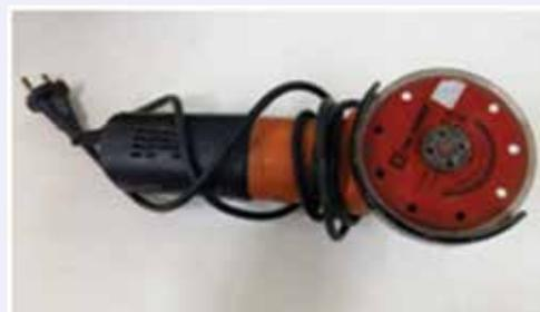
Fig. 2: View of a concrete saw cutting machine
