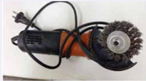
Fig. 9: Rebar cleaning equipment for removal of corrosion products of steel
