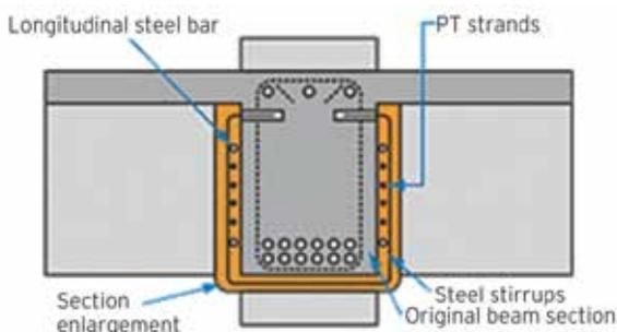
**Fig. 8:** Sketch showing strengthening of beam by section enlargement
