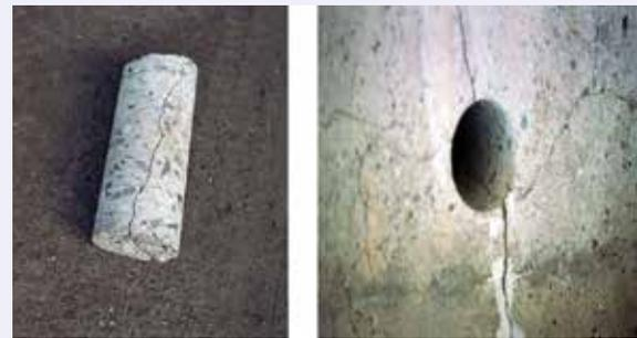
Fig. 7: Core sample taken from crack area
