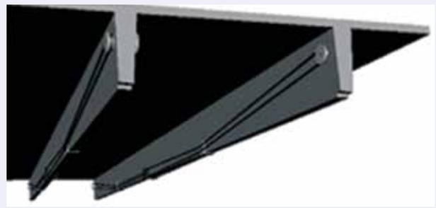
**Fig. 7:** View of external post-tensioning of beams
