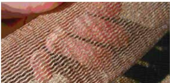
**Fig. 5:** 12WPI tape with cords held together by a polyester scrim for SRP composite bonding
