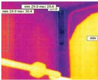
IR Thermography to detect delamination and voids of concrete and to find out the source of water leakage and location of water pipe
