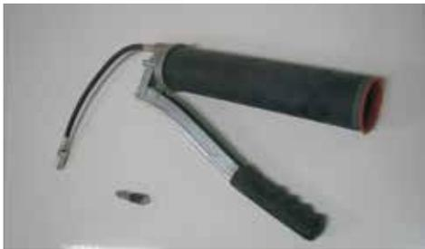
Fig. 2 a: Packer and Injection hand pump
