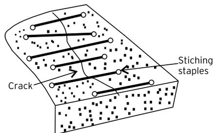
Fig. 3 : Stitching of cracks
