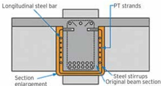
**Fig. 8:** Sketch showing strengthening of beam by section enlargement
