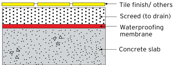
**Fig. 4:** Floor slab with waterproofing and membrane finishes
