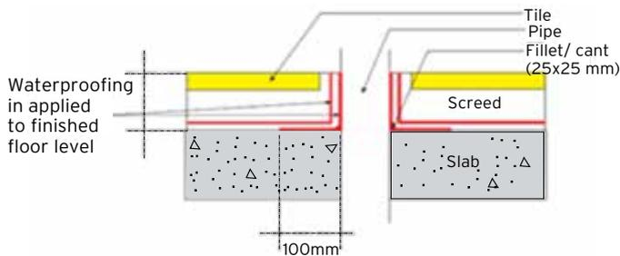
Fig. 14: Waterproofing details at floor penetration
