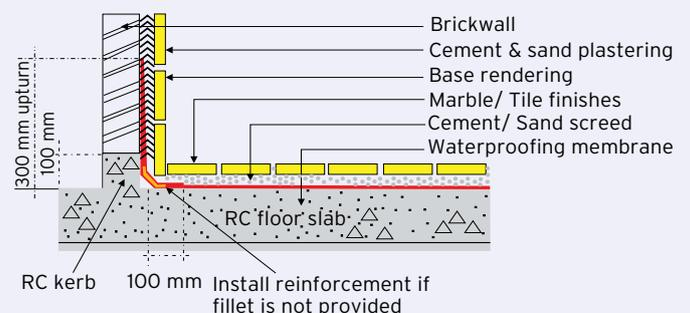
**Fig. 8:** Details on Waterproofing upturn at walls
