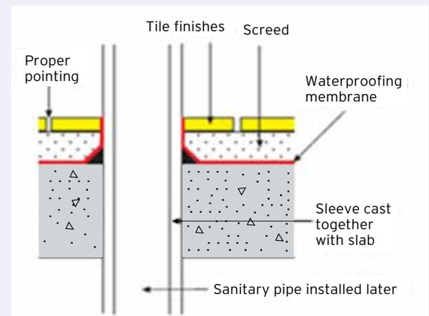
Fig. 13: Pipe sleeve cast with floor slab
