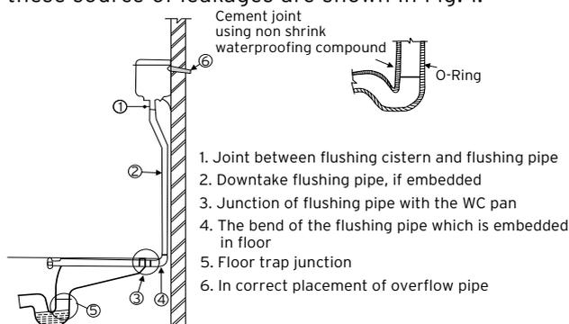
Fig. 1: Sources of leakages in WC & flushing cisterns
