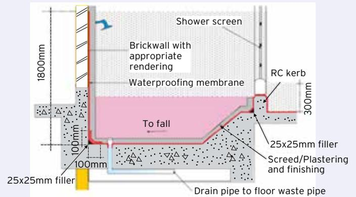
Fig. 12: Waterproofing details at sunken bath
