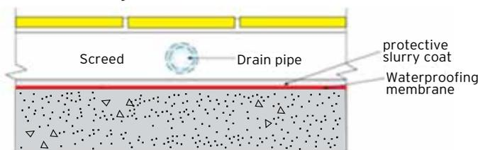
Fig. 16: Pipes embedded in screed
