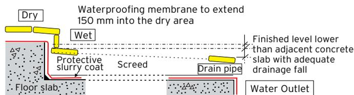
**Fig. 5:** Adequate drop in floor slab
