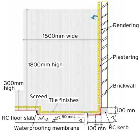
Fig. 9: Waterproofing details of shower area
