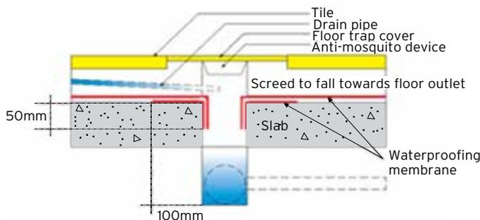
Fig. 15: Waterproofing details at floor outlet
